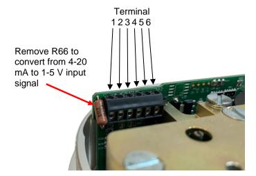
If the sensing resistor R66 is removed, we recommend placing a 10K resistor between signal and signal GND, or simply using shielded cables (for noise reduction).
